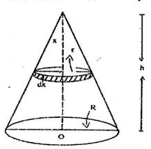
Therefore, the moment of inertia of the disc about the axis AO passing through its centre and perpendicular to its plane i.e.
