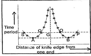
AB is determine from the graph. Once AB is found radius of gyration is calculated from the above formula.
