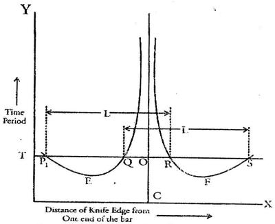
about any of these points is T. The pair of points P and R (or Q and S) are situated on opposite sides of the centre of mass C at unequal distances from it. So these points correspond to centre of suspension and centre of oscillation. The distance PR or QS is the length of the equivalent simple pendulum.
