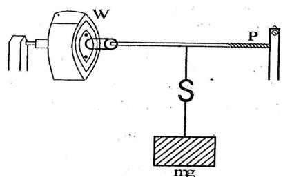
The loss of potential energy in dropping mass m through a distance h is mgh. This potential energy is used up in giving the kinetic energy to the system and against frictional work done i.e.
