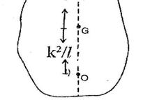
It shows that the time periods of oscillation about O and S are equal Hence, the centre of suspension and oscillation can be interchanged.
