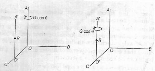
Hence, the system of forces acting on the rigid body is equivalent to a single force R acting along the line O'A' and a single couple of moment  $G\cos\theta$  about the same line O'A'. The axis O'A' is called poinsot's central axis and force R and couple of moment  $G\cos\theta=K$  together are called wrench and is written as (R,K).
