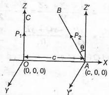
If (X, Y, Z, L, M, N) be the dyname of the given system, then X = 0 + 0 = 0.  $Y = 0 + P_2 \cos\left(\frac{\pi}{2} - \theta\right) = P_2 \sin\theta$  and  $Z = P_1 + P_2 \cos\theta$
